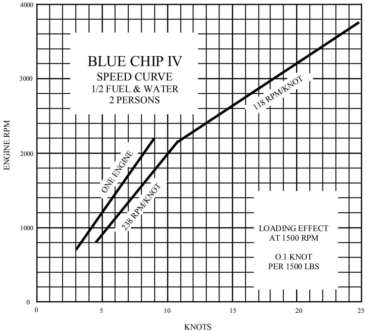
Round trip runs on the measured mile are made at each of several constant engine speeds, and the run each way timed by stop watch to the nearest second or better. At each constant engine rpm the speed measured in one direction is averaged with the speed in the other direction to cancel out the effect of current. The speeds, not the times, are averaged. The fuel, water, and crew load are noted. The results are plotted in the form shown.
